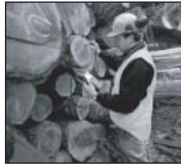
Log segregation based on wood stiffness: "Hitman" tool, developed by Industrial Research and Carter Holt Harvy (New Zealand)
