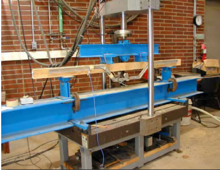
Figure 1. Demonstration of lumber testing at the 2005-06 PNWTIRC Annual Meeting, OSU Dept. of Wood Science and Engineering. A force of 500 pounds is applied to the center of a supported beam, and lumber deflection is measured to estimate wood stiffness.
